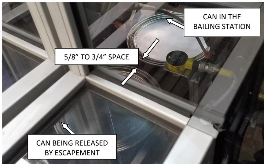
Adjust the escapement photo eye bracket downstream for more space, and upstream for less space.
